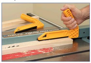
Also featured on these push sticks is the foam lined base. This helps provide you with even more control while feeding the stock through the blade. It also prevents slipping which can sometimes occur with standard style push sticks.
