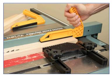
When used with a featherboard, the push stick becomes even more useful. The sideways pressure from the featherboard, along with the push stick from behind the stock provides the user with a safer more efficient way to cut narrow stock on a table saw.
