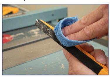
Before each use, inspect the foam pad on the bottom of the push stick. Make sure it is clean and debris free. We recommend using warm water on a cotton or micro-fiber cloth to wipe the pad clean. Make sure pad is completely dry before using.
