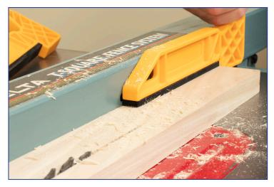
This push stick has a 90 degree notch with a relief circle cut out. This helps "hook" the back end of your stock much better than standard styles of push sticks.
